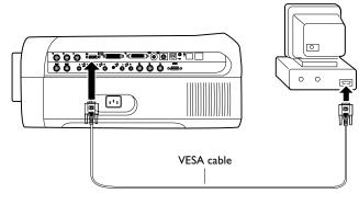
**NOTE:** If you are connecting an older Macintosh computer that has a 2-row 15-pin connector, you must use a Mac adaptor between the computer and the projector. See "Optional Accessories" on page 50.
